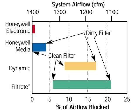
Testing was conducted in laboratory and actual homes by measuring total system airflow with various clean and loaded filters. Average results are reported. Results may vary depending on the characteristics of the blower. Filtrete® is a trademark of 3M Corporation.
