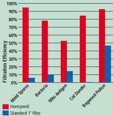
Independent testing<sup>2</sup> shows that Honeywell Electronic Air Cleaners capture a very high percentage of mold spores, bacteria, dust mite antigen, cat dander and ragweed pollen from the air that passes through the filter. The Honeywell Electronic Air Cleaner captured more than 90% of mold spores and ragweed pollen from the air passing through the air cleaner, more than 70% of bacteria and cat dander, and nearly 60% of dust mite antigen.
